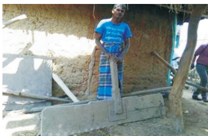
Parambu and Kodinjal for Sathuram adithal / leaveling and bunding in slopy lands
