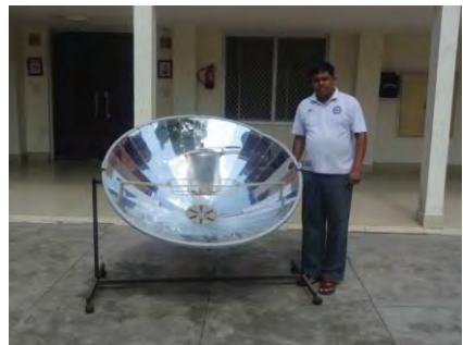
Parabolic Solar Cooker installed in Officers' Mess for reduction of LPG consumption
