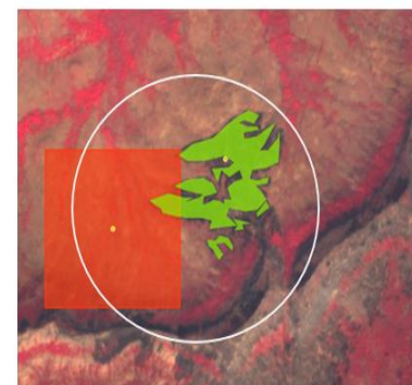
Post-Fire Satellite Image overlaid with MODIS pixel (red) and digitized burnt scar polygon (green)
